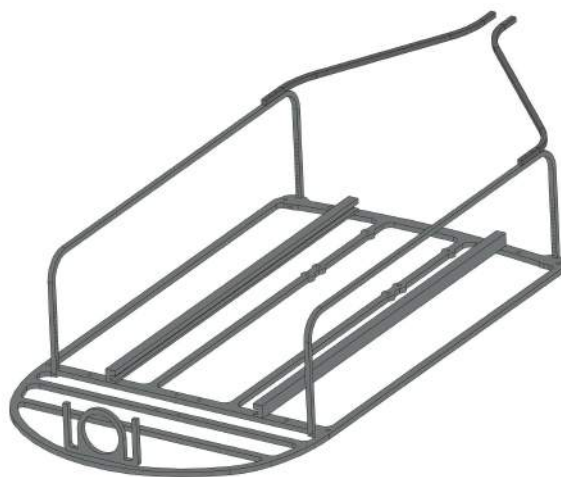
Fig. 1. SubmURSA frame with uprights and IMU arms
