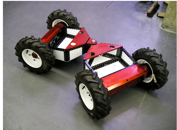
Figure 1: Completed URSA mechanical platform
