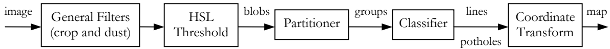
Figure 8: Vision system flow from camera images to a real-world coordinate map of features around the vehicle
