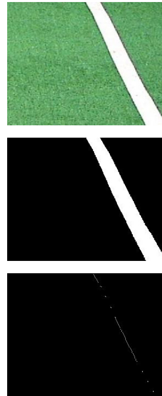
Figure 12: (from top) original image, histogram thresholded image, line identification
