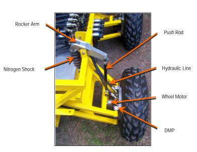
Figure 1 – Mechanical detail.
