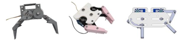
SIMPLE and MEDIUM designs are well known/common mechanisms, and little was done to improve them during development and prototyping. Whereas the COMPLEX mechanism encountered a fatal flaw in design at prototyping: the pins would get stuck and not move smoothly, and/or the pincers would rotate and not remain perpendicular to the slot/track.
