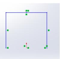
Use the smart dimension tool to set the dimensions of the sketch, select the feature you want to dimension (typically a line or pair of points) to bring up the dialogue box. To use global variables for dimensions, simply type "=" in the dialogue box and hover over global variables.
