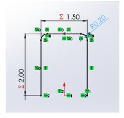
Lastly, add a 0.20in radius fillet to each of the two top corners using the sketch fillet feature.
