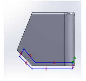
To link the base thickness dimensions, CTRL and select both of the  $\frac{1}{8}$ " dimensions then right click and select link values. Name the linked dimension Base Thickness.
