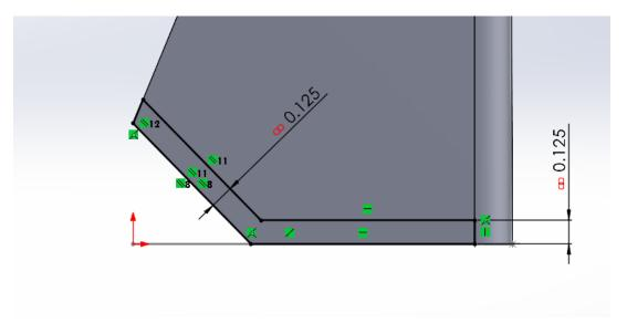
To finish off the extruded boss, choose Extrude to Surface for both directions and select the inner faces of the bin as shown
