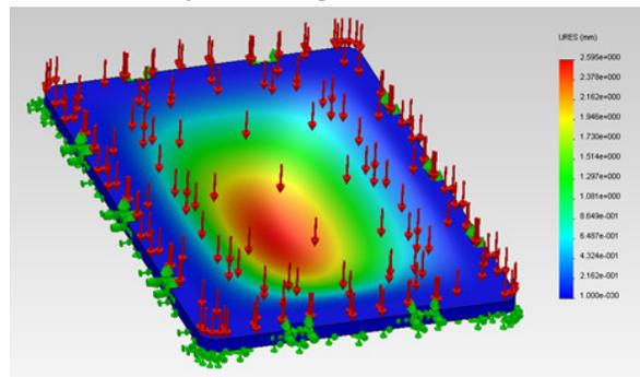
**Figure 5: Simulated deflection mapped over lid at 10 m.**
