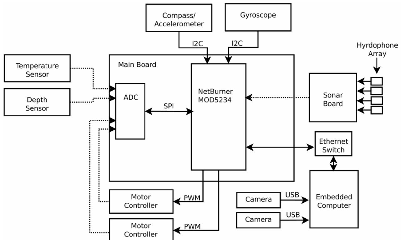
**Figure 1: Overview of electrical systems used in SubmURSA.**
