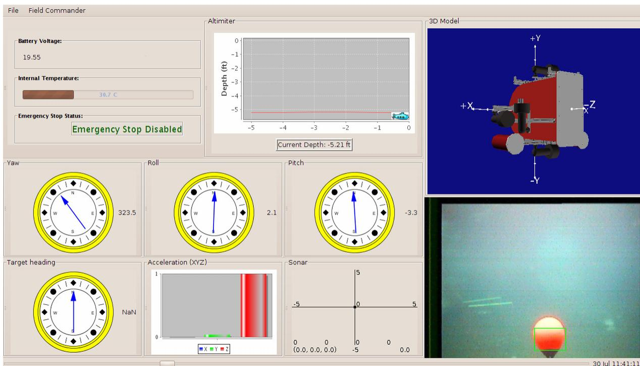
Figure 3: Screen capture of graphical display / remote control interface.
