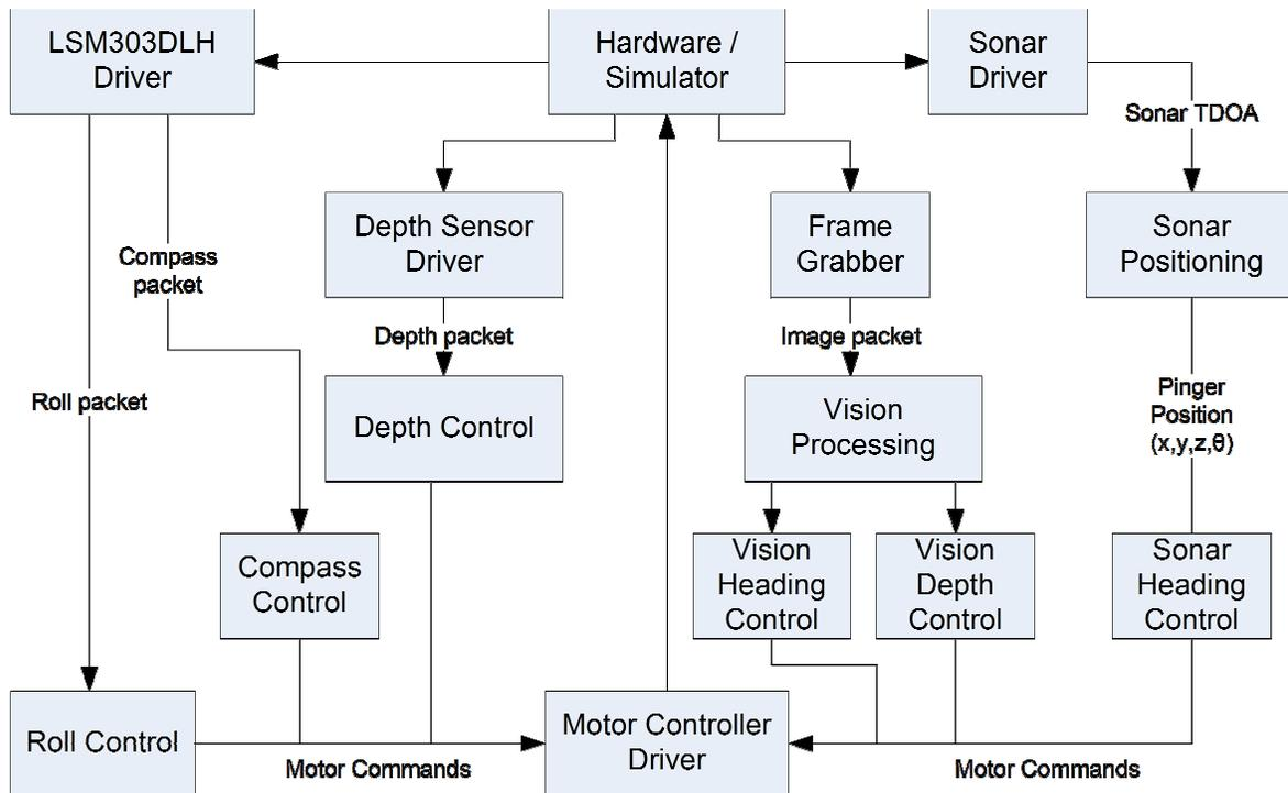
Figure 2: Overview of SubmURSA's software components.
