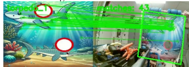
Figure 3. Feature matching between the reference image (left) and the camera feed, with lines drawn between identical features; 43 matches are shown for object localization.
